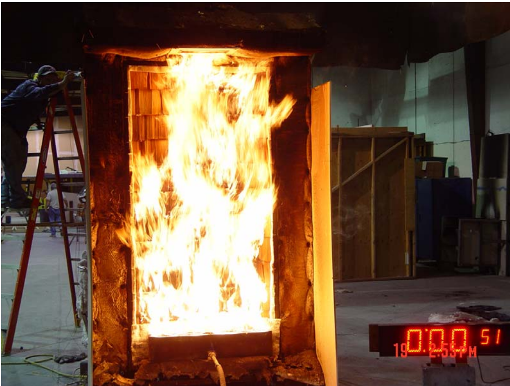
Flame intrusion exposure
