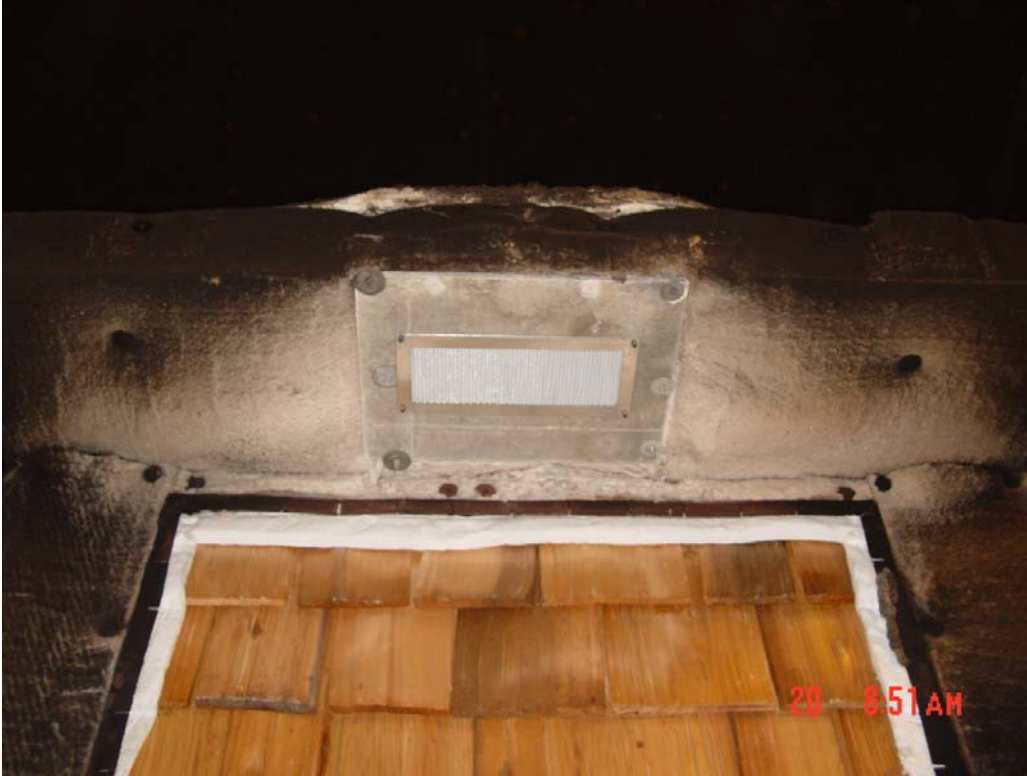
Vent in position prior to flame exposure
