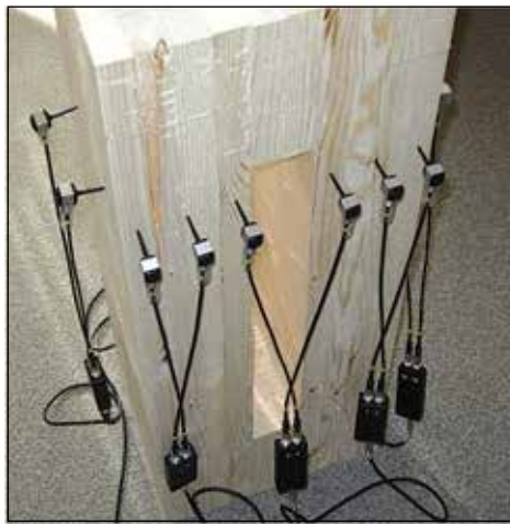
Figure 4.3—Acoustic tomography test on a glued-laminated specimen with a simulated void (Divos 2006).
