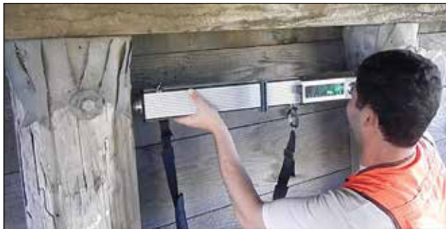
Figure 2.13—Electronic display on a resistance drill.
