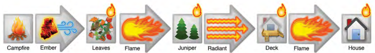
Figure 4-1: Professionally rendered prototype fire pathway depicting ember ignitor to home ignition. This fictional pathway example depicts embers generated by a campfire being carried by wind and igniting dry leaves that spreads flames to nearby juniper shrubs which, in turn, are located near enough to ignite a wooden deck by radiant heat which ultimately spreads fire to a home.
