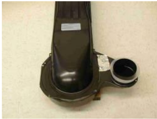
(a) Blower removed from the dryer
