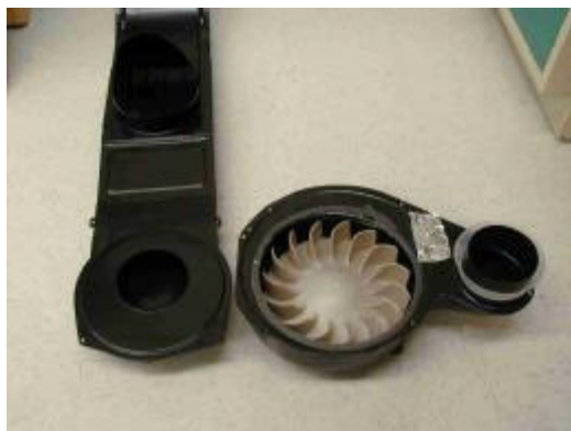
(b) Blower housing separated
