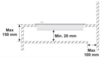
IMPORTANT: if the appliance is mounted on a unit, make sure that a separating shelf is installed, as shown in the figure.
