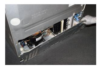
PHOTO: Remove the back panel.
