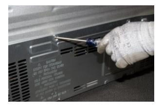
PHOTO: Remove the back panel screws.
