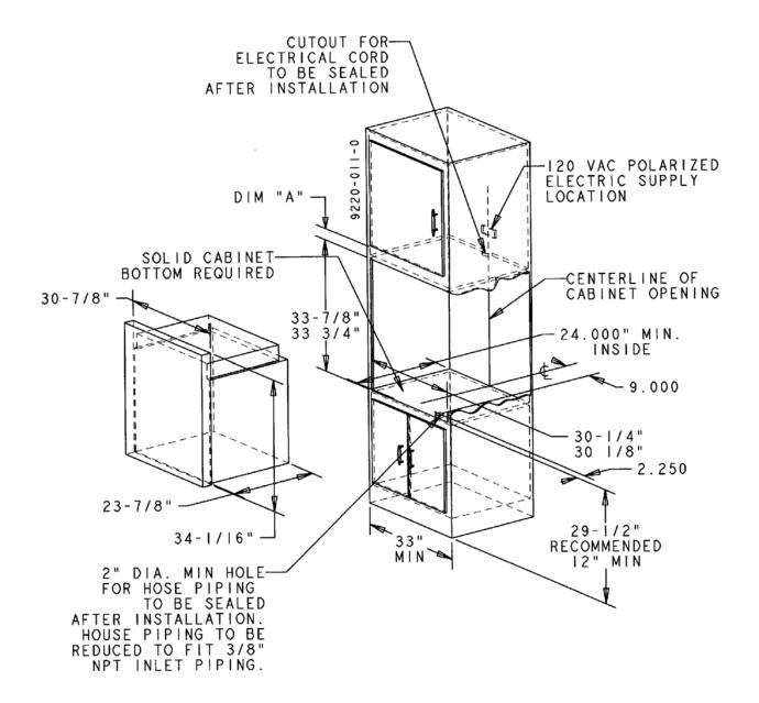
**DIM A:** If cabinet doors are provided above the gas wall oven, a minimum spacing of 3-3/4" is required for 1/2" thick doors. Thicker doors required an additional 1" (inch) added to the 3-3/4" for each 1/4" additional thickness.
