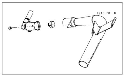
**Exploded Bottom Burner Assembly**
