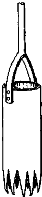
Fig. 42 Fishing tools. (c) spear for retrieval of broken rope or cable with latch for picking up bits or bailers
