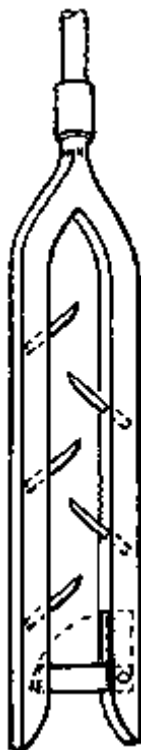
Fig. 42 Fishing tools. (d) hook with guide for attaching supplemental line to stuck tool
