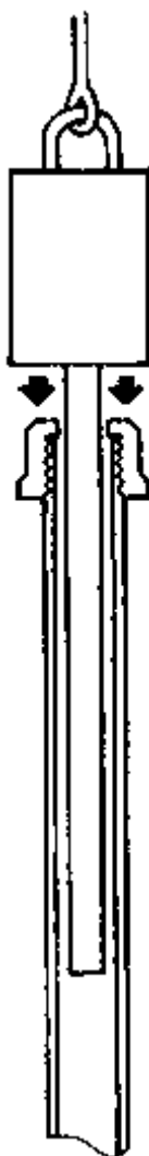
Fig. 13 Devices for well driving. (c) driving on clamp
