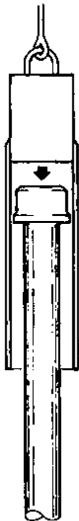
Fig. 13 Devices for well driving. (a) guided on outside of pipe
