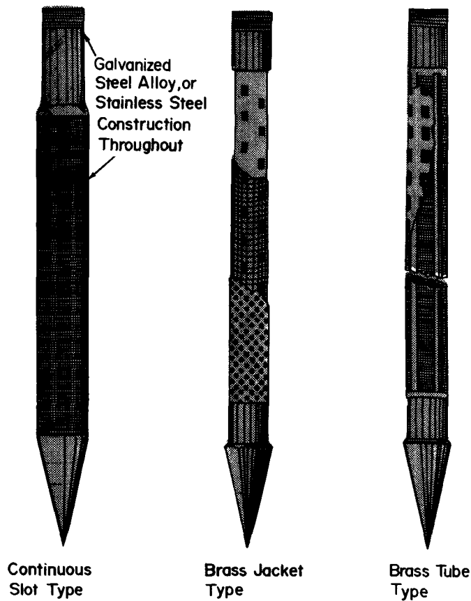
FIGURE 4. - Different kinds of drive-well points.
