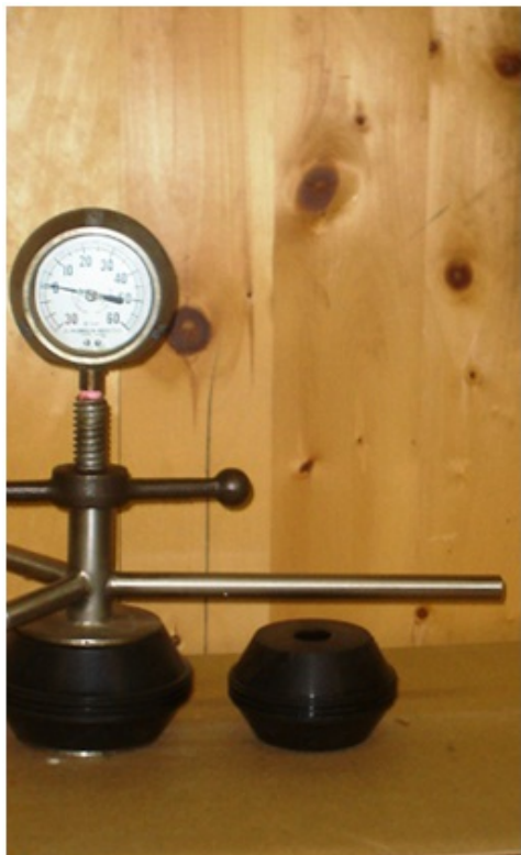
Figure 12-5: Flowing Well Pressure Gauge Device - Installed
