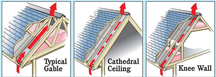
Maintaining an unrestricted air passageway between the soffit and ridge is crucial to the performance of the vent system, and must not be blocked or restricted. COR-A-VENT recommends a minimum 2" air space between the roof sheathing and vent chute or insulation
