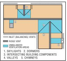
*b) vent opening* (sq. in. net free vent area/NFVA) in the soffit (intake) than at the ridge. For example, our V-300 products have 13.5 sq. in NFVA per lineal foot. To balance this, you need 2 soffit/eave/intake vents of at least 6.75 sq. in. per lineal foot (1/2 of 13.5 in each overhang).
