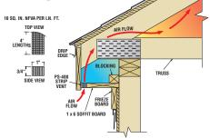
Another new soffit product from COR-A-VENT is the **PS-400 Strip Vent**, a <sup>3</sup>/4" wide continuous strip that's perfect for 1x soffit panels. Like the original Strip Vent, PS-400 is available in either black or white and provides 10 sq. in. Net Free Vent Area per lineal foot. Pre-attach **PS-400** to the 1x for quick installation.
