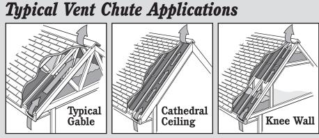
Maintaining an unrestricted air passageway between the soffit and ridge is crucial to the performance of the vent system, and must not be blocked or restricted. COR-A-VENT recommends a minimum 2" air space between the roof sheathing and vent chute or insulation
