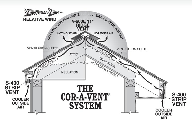
A balanced vent system is one that best utilizes three natural forces: air pressure, the thermal effect and diffusion. Basically, for every square inch of ridge (exhaust) vent you must balance it with **at least one square inch or more of soffit (intake) vent.**
