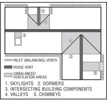
free vent area/NFVA) in the soffit (intake) than at the ridge. For example, our V-600 products have 20 sq. in NFVA per lineal foot. To balance this, you need 2 soffit/eave/intake vents of approximately
