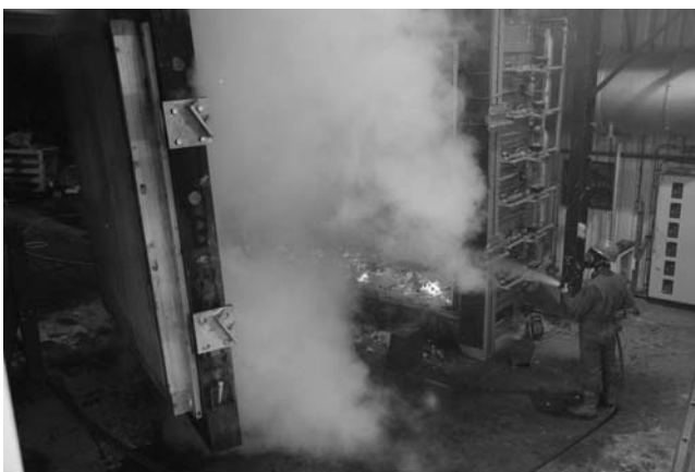
Figure 5. Panel being removed from furnace after fire test (Chiltern International Fire, 2009)
