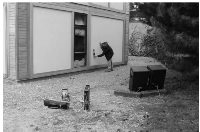
Figure 6. Sound insulation performance test being conducted on prototype house
