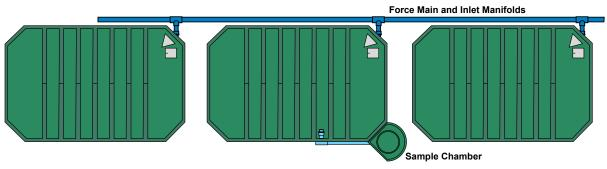
Blue coded modules with weep holes and one green coded module with sampling chamber, drain into a stone pad for final treated effluent disposal. Pad dimensions can be selected to match site conditions and modules can be installed side-by-side as well as end-to-end (as shown above)
