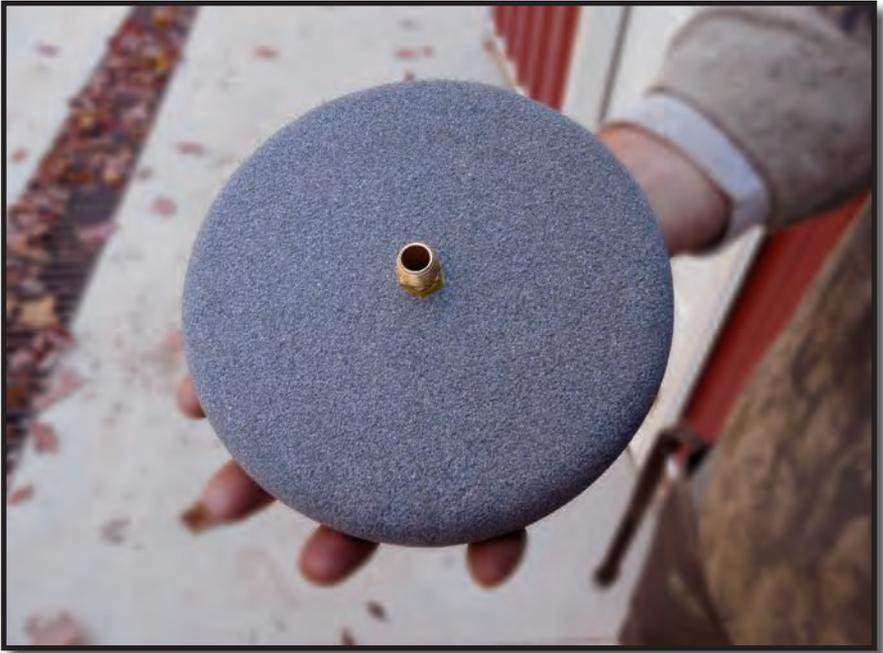
The airstone is a hard stone-like disc that have fine holes all through it. As the air passes through the stone, the air breaks down into a fine mist of air bubbles. As the bubbles rise to the surface, some of the oxygen on the air will be trapped in the water. Also, the windmill will keep a circle of water open even in the coldest part of winter, therefore providing a place for ducks to swim and protect themselves from predators.
