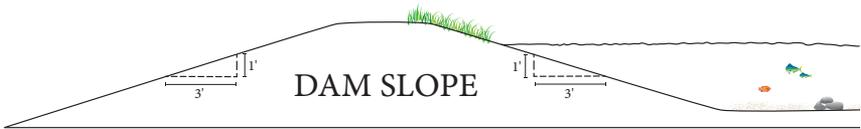
*The illustration above shows the 1 to 3 slope of the dam.*
