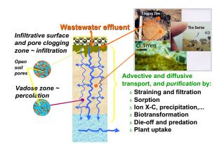
Fig. 2. Illustration of wastewater soil absorption system treatment processes.
