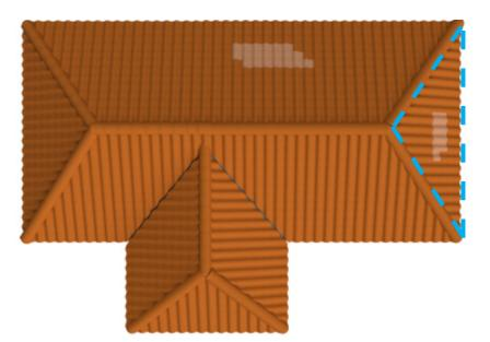
Plane or roof area that was removed and installed with new tiles. (when similar tiles)
