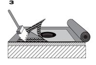
**3** Apply solvent welding agent every 50 mm to both sides of the seam region, and press down by hand. Then load the seams (e.g. with a sandbag). When using hot gas welding, close the seam with the hot gas hand-welding unit and pressure roller or with a welding machine.
