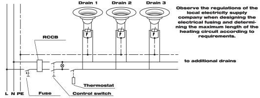
Heated roof drains can be connected individually or in parallel.
