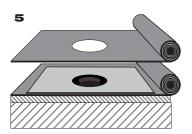
**5** Unroll the **top** sealing sheet over the drain. Cut a circular hole in the sealing sheet in the region of the drain – hole diameter approx. 150 mm.
