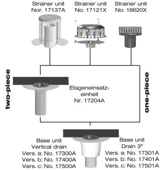
Vers. a = without thermal insulation, vers. b = with thermal insulation, vers. c = with thermal insulation and heating
