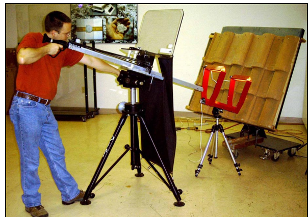
Figure 1. Ice ball launching (IBL-7) device with light sensors (chronograph) developed for impact testing.
