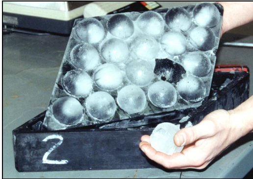
Figure 2. Solid ice balls made in rubber molds were utilized for impact testing on roofing products.
