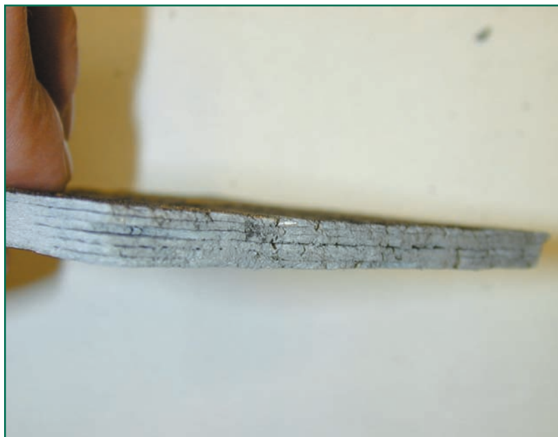
Photo 5 – Cohesive failure of the laminates
