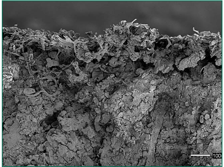
Photo 8 – SEM Image (original mag = x100) of cross-section of surface of fiber-cement sample taken from area colonized by Scytonema
