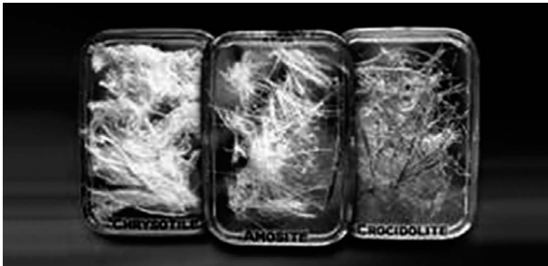
Figure 4: Three commonly found forms of asbestos are chrysotile, amosite and crocidolite.
