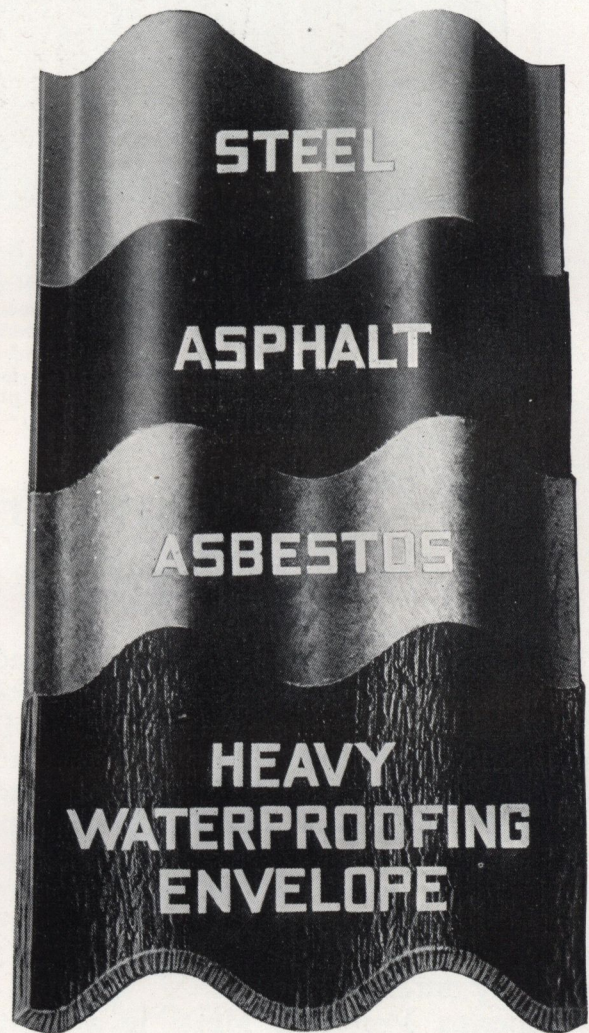
Sample of Asbestos Protected Metal with portions cut away to show relative position of the three corrosion-proof and insulating coatings with steel base or core.
