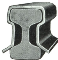
Wilgus Under-running third-rail covered with indurated fibre covering.
