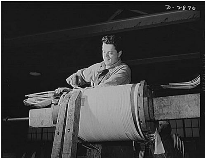
Figure 5. Worker winding an asbestos insulated low-volt coil (1942). Photographer: Alfred T. Palmer. Library of Congress Prints & Photographs Division.
