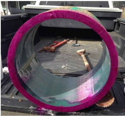
Phenolphthalein Dye Test
