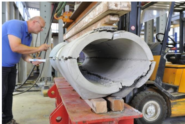
Crushing Strength Test
