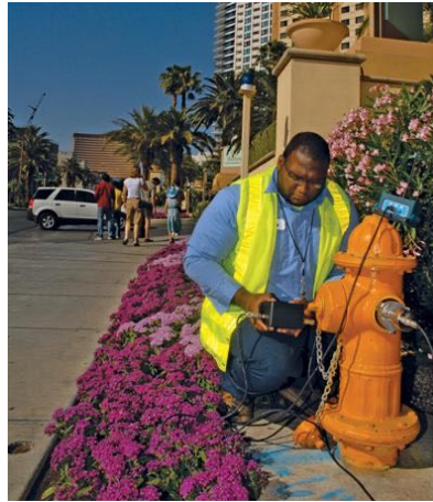
Acoustic Velocity Test
