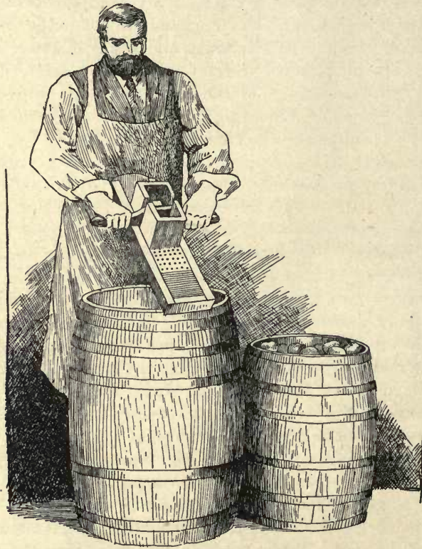
FIG. 3.—Primitive apple grater in use in Germany.
