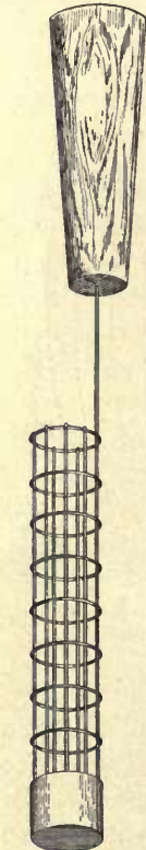
FIG. 22.—Device for burning sulphur match in casks.
