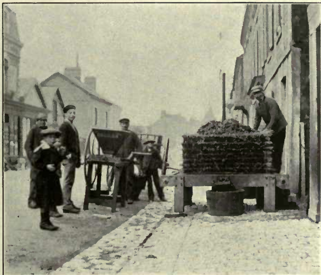
FIG. 1.—ITINERANT CIDER MAKERS AT WORK IN STREETS. STRAW USED IN BUILDING UP CHEESE, RENNES, FRANCE.
