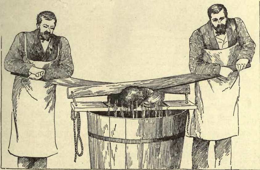
FIG. 5.—Primitive double-lever cider press in use in Germany.
