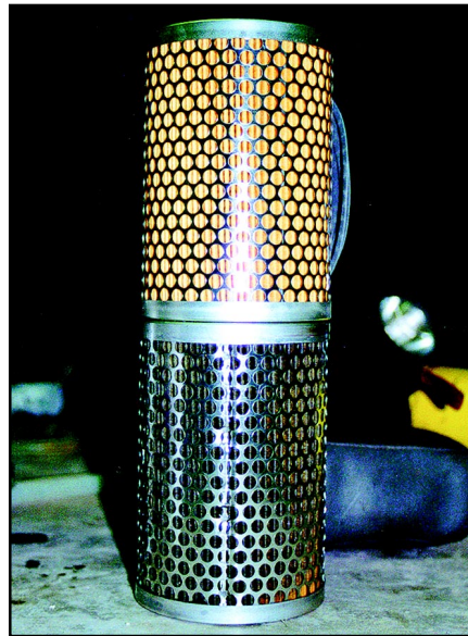
Figure 2: Clean (top) and dirty (bottom) refrigerant suction line filters.
