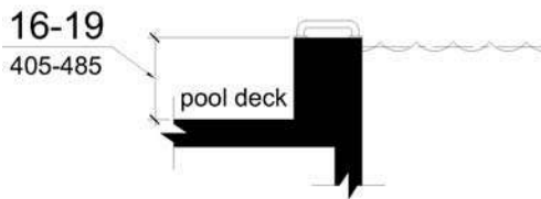
Fig. 75 Transfer Wall Height
